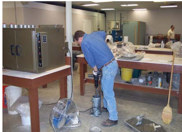
Figure 4 – Preparation of a Strength Test Cylinder using a Vibratory Rammer
