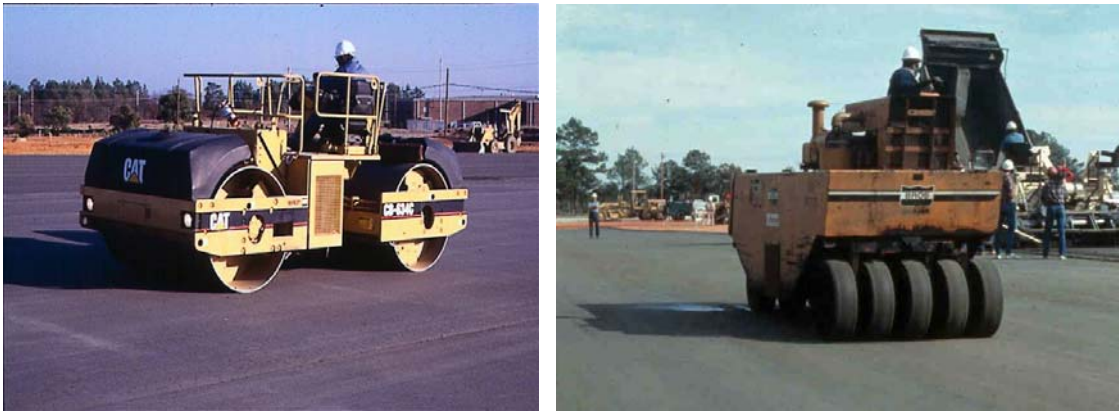
Figure 6 – Examples of a Vibratory Roller and a Rubber-tire Roller
